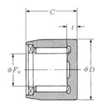
NSA04002 Bearing 2D drawings and 3D CAD models
